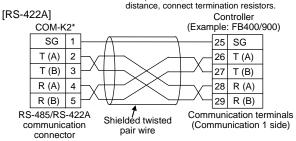
\* The termination resistor is built into the COM-K2.
