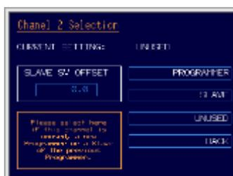
On the “Channel selection screen” you can select each channel to be a programmer, slave of the previous programmer or unused, by pushing the corresponding button. You can go back to the previous channel at any time, by pushing “BACK” button.
