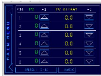
Push the “PV OFFSET” button to swap to the calibration screen. On the calibration screen the operator can add or subtract some degrees of the process values to calibrate the controller with your paper trend chart recorder. Touch the number to set the value by the pop-up keypad. Touch the up and down keys to directly add or subtract one. Push the reset screen to “zero” the applicable channels. Push “BACK” to return to the main menu.
