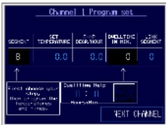
On the profile setting screen, there are four parameters that can be set for each segment. First select the segment you want to set by touching the segment number. The keypad will pop-up and you can select the segment you want to program, from segment 1 to segment 8. Always start your program in segment number one!
