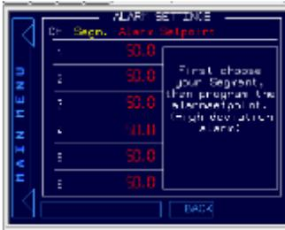
You can set a alarm per channel per segment. To do so, first select a segment from which you would like to set an alarm and then select the alarm column. You can insert a minimum of 0.0 degrees deviation high alarm, and a maximum of 1200.0 degrees.
