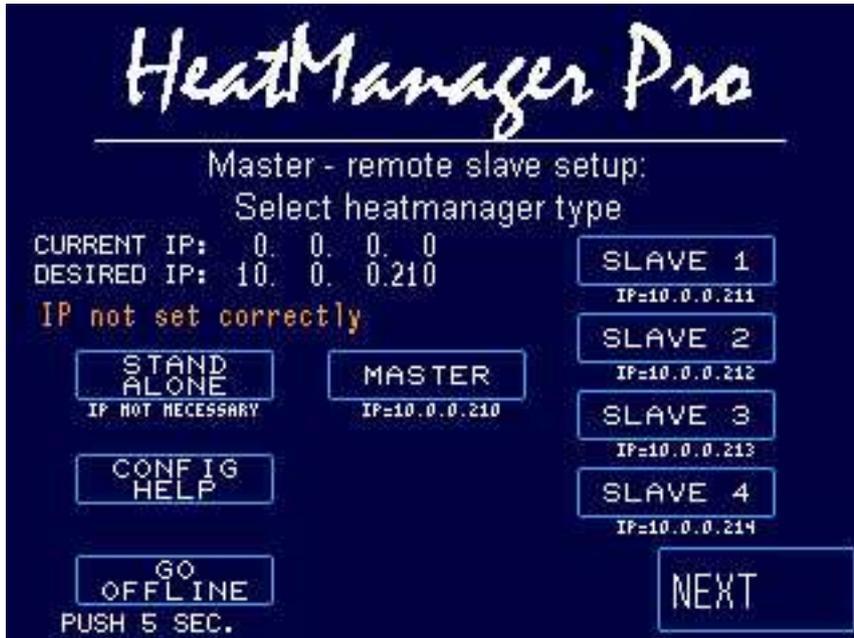
This screen comes up when you configure the master-slave configuration. Put the heatmanager back to stand-alone if it needs to operate without the slaves again, otherwise you will get communication errors.
