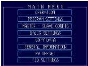
From the main menu you can choose to go to the Operation mode, the Program settings, Master-Slave interconnection configuration, Basic settings, Copy data, General information, PV offset and PID settings.
