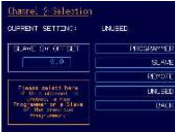
On the “Channel selection screen” you can select each channel to be a programmer, slave of the previous programmer, remotely controlled by another master-heatmanager or unused, by pushing the corresponding button. You can go back to the previous channel at any time, by pushing “BACK” button.
