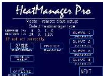
The stand-alone mode is used if the Heatmanager does not have to be interconnected to other heatmanagers. Please select this option because if you set it to master or slave, it tries to interconnect to other heatmanagers, so only set it to master- and or slave when this is necessary.
