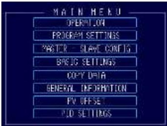
Push the “OPERATION” button in order to swap to the operations menu where you can RUN and STOP one or all of your programmers by pushing the corresponding channel number button. For each channel the “P”, the “S”, the “R” or the “U” indicates whether that channel is a Programmer, Slave, Controlled by a Remote Heatmanager or set to Unused. Programmers can easily be recognized by their blue rectangle surrounding the channel number.
